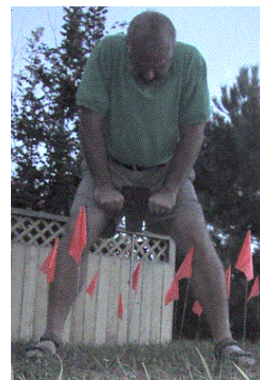
Figure 3: Author pushing soil compaction meter into the ground.
