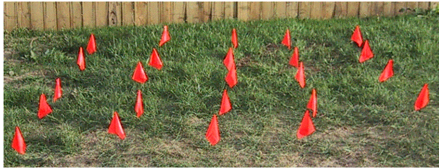
Figure 1: 2-meter x 2-meter area with survey flags positioned at 0.5-meter grid intervals.
