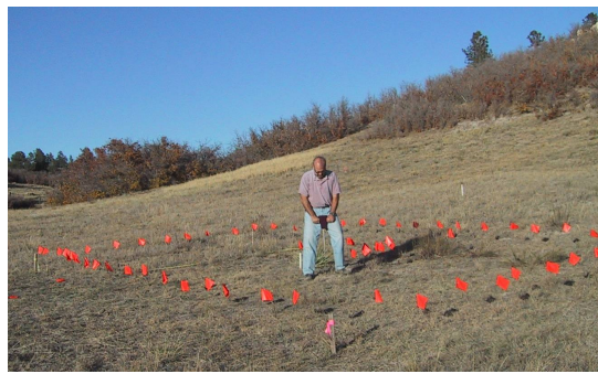
Figure 11: Sampling a 8 x 6 meter area at the NecroSearch research site (buried pig depicted by flagging upslope from author's left foot).
