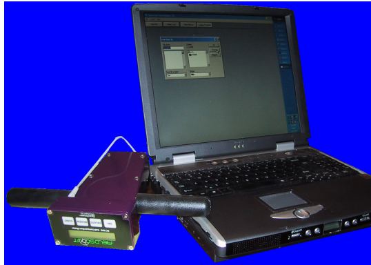
Figure 4: Spectrum Technologies Field Scout Model SC900 soil compaction meter connected to laptop computer via a serial cable.
