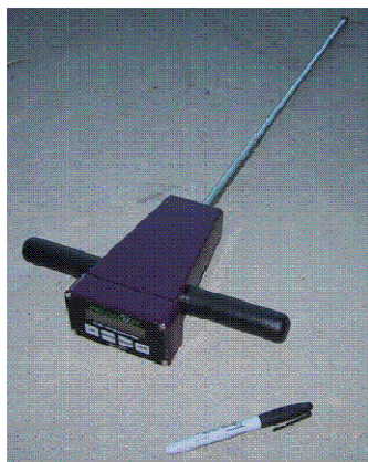
Figure 2: Spectrum Technologies Field Scout Model SC900 soil compaction meter.
