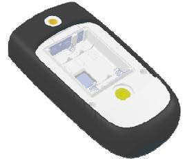
**Warning!** Do not connect the meter to the power adaptor or to a USB when non-rechargeable, alkaline batteries are installed. This may damage the batteries and/or meter.
