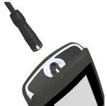
**Note:** Do not turn the probe connector once inserted into the meter's socket. When removing the probe, pull on the connector, not the cable.
