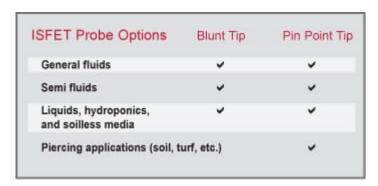
Uses patented non-glass ISFET technology for general purpose pH measurement
