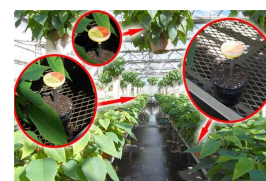
Position the meters throughout your location and compare differences in light levels and the effect on plant growth and quality
