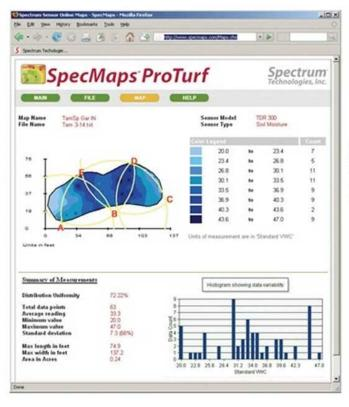
SpecMaps ProTurf brings in the ability to show sprinkler head locations and Distribution uniformity. This works with the FieldScout TDR 300 only
