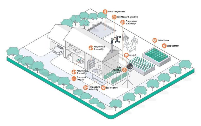
Sensor Transmitters are the building blocks of your custom network of sensors. They can be positioned indoors or outdoors and are capable of transmitting data up to 1,000 ft. (300 m). Each transmitter can support up to five sensors, including an Anemometer, Rain Collector, Temperature Probe or Temperature & Humidity Sensor, UV Sensor and Solar Radiation Sensor.
